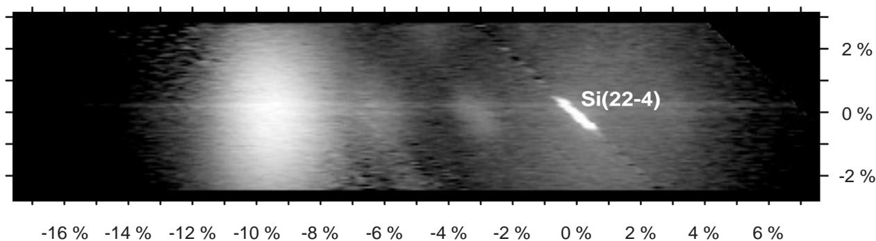
Figure 1: Reciprocal space map for  $q_z \simeq 0$  for a 5 nm thick Ge film. The bright spot is the  $\text{Si}(22\bar{4})$  Bragg peak, the diffuse broad spot is the  $\text{Ge}(22\bar{4})$  Bragg peak. Four satellite spots originating from the periodical dislocation network at the Ge/Si interface are found in between the Si Bragg peak and the Ge Bragg peak.
