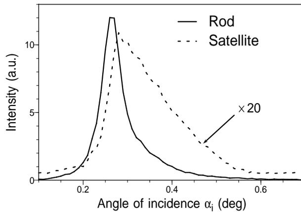
Figure 2: Rodscan of fundamental spot and satellite spot. Due to the finite vertical extension of the strain fields intensity is still observed for larger vertical scattering vectors  $q_z$
