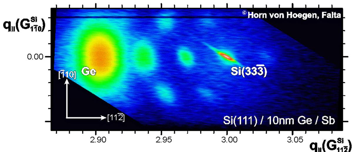
**Figure 1:** Heterosystem with 10 nm Ge(111) on a Si(111) substrate. In-plane scan of (33-3) Bragg condition. Satellite spots due to interfacial dislocation array are visible
