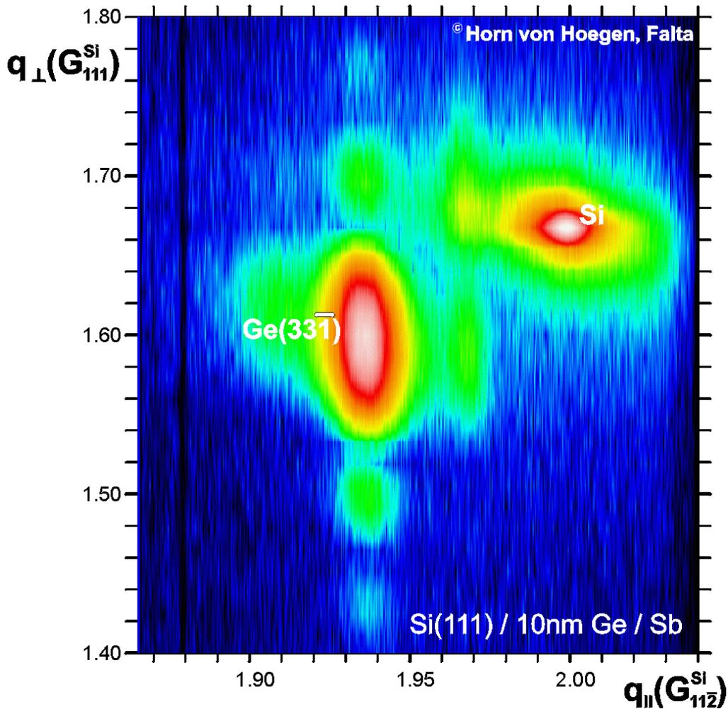
**Figure 2:** Vertical cut of reciprocal space at the Ge(331) Bragg condition. Both Si and Ge spots are visible. Satellite spots surround the Ge and Si spots.
