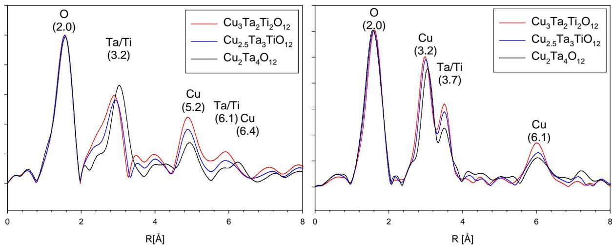
Figure 1a:  $FT(\chi(k) \cdot k^3)$  Cu-K EXAFS of Ti doped samples.
